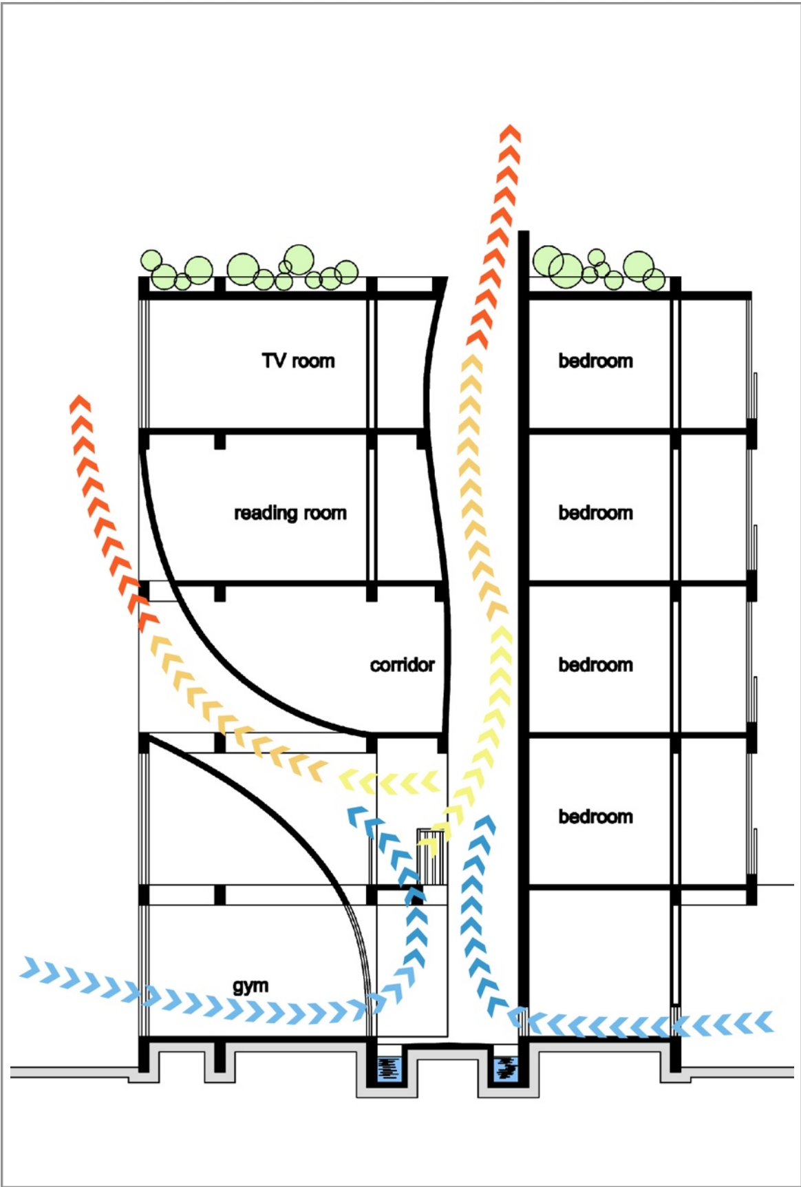
Figure 73: Diagram of Passive Ventilation in Scoops
